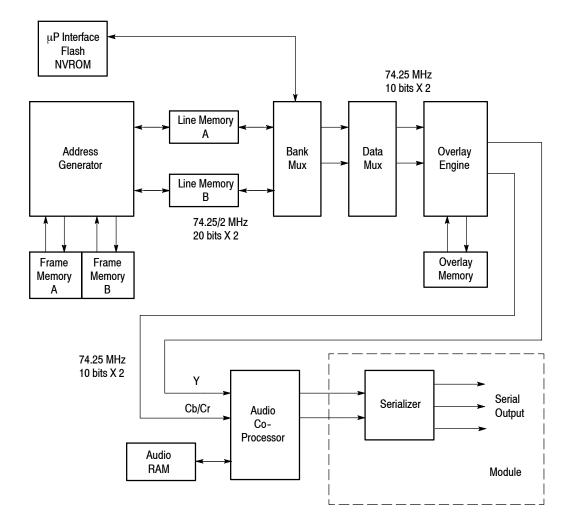
Figure 3-1: Simplified block diagram of the HDVG1 Generator module
