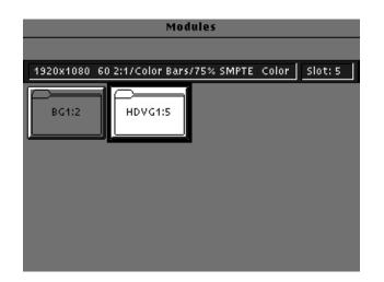
6. Touch the module icon on the display (or push the **Signal Sets** button if the desired icon is already highlighted). The installed signal sets for the module appear. Selections you make after this will pertain to the HDVG1 Generator module.
