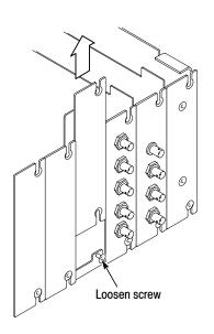
5. Remove the appropriate rear panel as shown in Figure 2-3. Loosen, but do not remove the bottom screw. You will use it later to secure the module.
