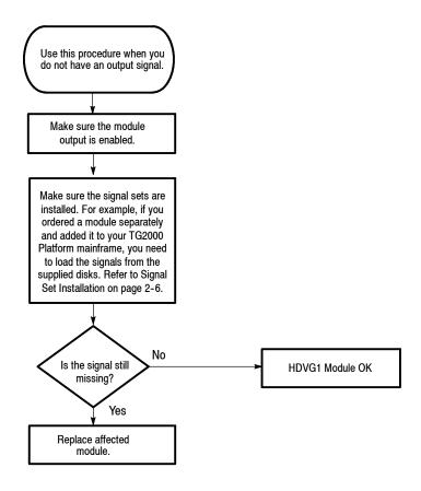
Figure 5-10: Flowchart for missing output signal
