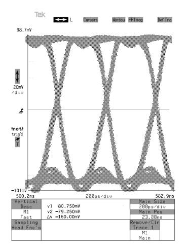
2. Check that OUTPUT 1 eye pattern displayed on the sampling oscilloscope is fully open. Figure 4-3 shows an example of the eye pattern for an acceptable output signal
