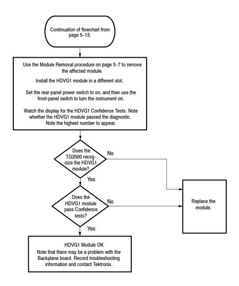
Figure 5-5: Flowchart for checking the module in a different slot
