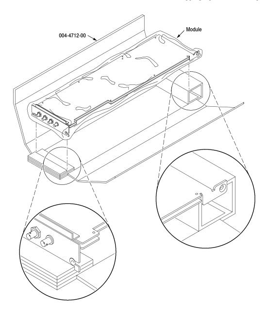
Figure 5-1: Placing the module in the protective wrapping
