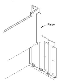
Figure 2-4: Module flange
