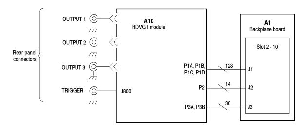
Figure 7-1: HDVG1 Generator module connections
