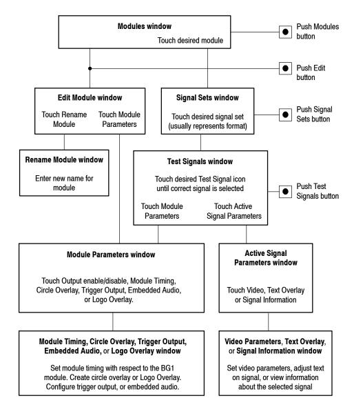
Figure 2-7: Menu structure for the HDVG1 Generator module
