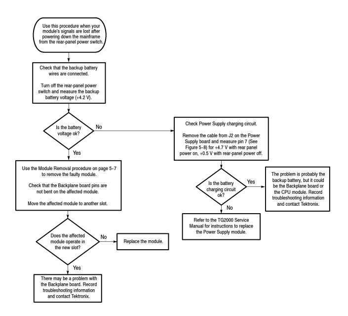
Figure 5-7: Flowchart for signals lost after power down
