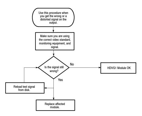
Figure 5-9: Flowchart for wrong signal on output
