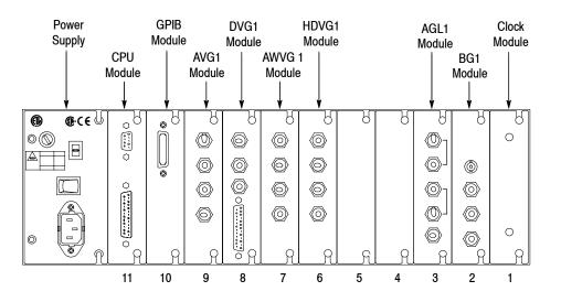
Figure 2-1: TG2000 Platform mainframe rear panel, showing slot numbering
