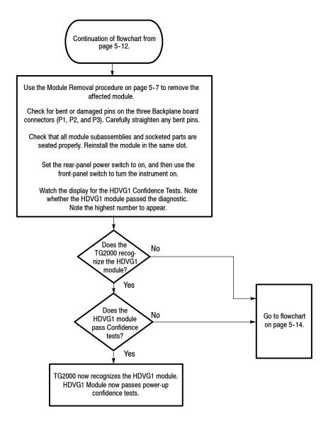
Figure 5-4: Flowchart for checking the current module installation slot
