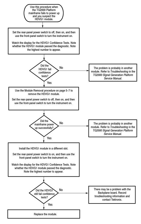
Figure 5-6: Flowchart for failure to power up
