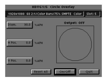
If you want to reset the values, touch **Reset All**. This will set the diameter, horizontal, and vertical to 90%, 0, and 0 respectively.
