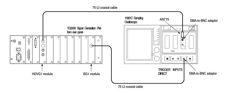
Figure 4-2: Eye pattern check connection
