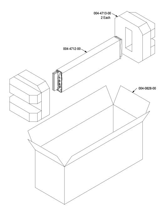
Figure 5-2: Placing the module in the shipping carton
