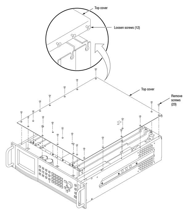
Figure 2-2: Top cover removal
